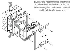
**SIGA-MAB:** mount the UIO motherboard inside a suitable ED-WARDS enclosure with screws and washers provided. Plug the module into any available position on the motherboard and secure the module to the motherboard with the captive screws. Wiring connections are made to the terminals on the motherboard (see wiring diagram). UIO motherboard terminals are suited for #12 to #18 AWG (2.5 mm² to 0.75 mm²) wire size.
