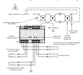
Max. 12.5 ohms resistance per wire for Class A configurations.
